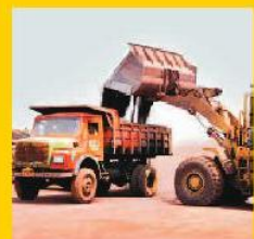
Loading of coke
